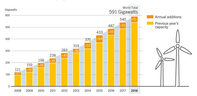
FIGURE 35. Wind Power Global Capacity and Annual Additions, 2008-2018
