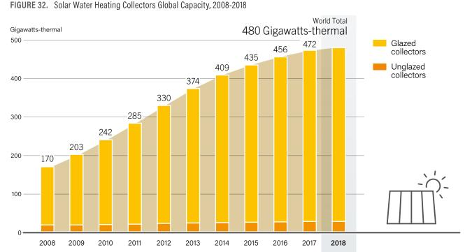
Note: Data are for glazed and unglazed solar water collectors and do not include concentrating and air collectors.
